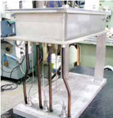
Flat type Heater designed for hazardous environments
